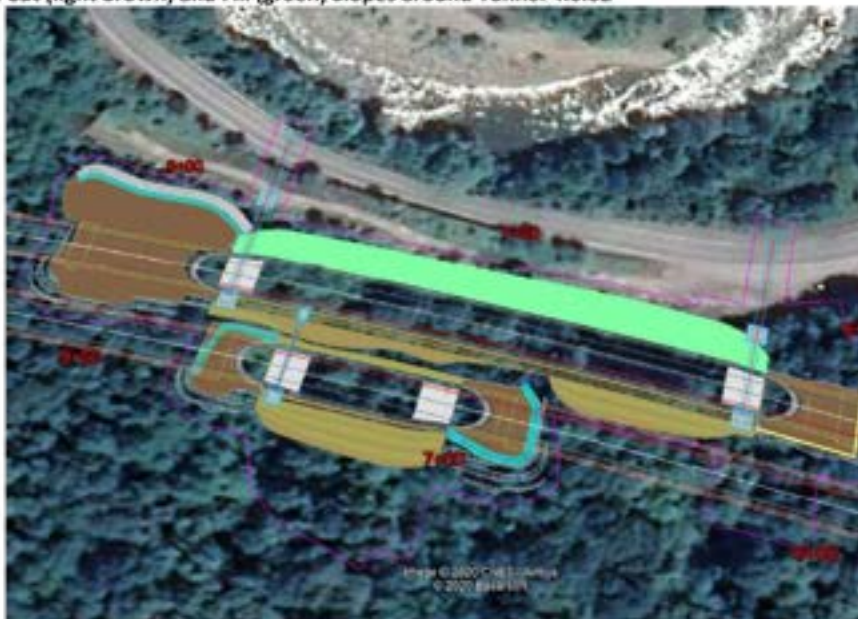
Figure 1: Cut (light brown) and Fill (green) Slopes around Tunnel 4.0.02
