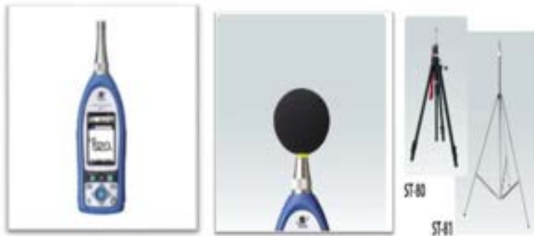
Figure 3-3 Noise monitoring equipment
